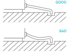
1 Attach the free end of inlet hose to the water supply tap (see image 4).Hand tighten sufficiently to provide leak free joint. It is advisable to have the stop valve within easy reach.
