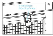
Notice: The screw position of icethickness sensor determines the distance between the sensor reeds and evaporator plate. Delux stanard gap space should be range of 4mm-7mm, please keep gap space properly.
